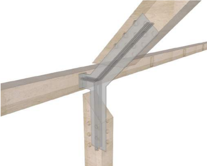
Eaves portal connection
